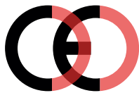
False CE Mark (too close)
