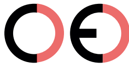
False CE Mark (too far)
